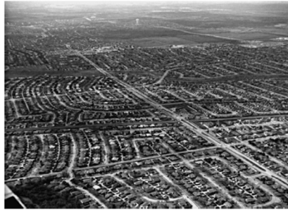
EXPOSURE B SUBURBAN RESIDENTIAL AREA WITH MOSTLY SINGLE-FAMILY DWELLINGS. STRUCTURES IN THE CENTER OF THE PHOTOGRAPH HAVE SITES DESIGNATED AS EXPOSURE B WITH SURFACE ROUGHNESS CATEGORY B TERRAIN AROUND THE SITE FOR A DISTANCE GREATER THAN 1500 FT OR TEN TIMES THE HEIGHT OF THE STRUCTURE, WHICHEVER IS GREATER, IN ANY WIND DIRECTION
