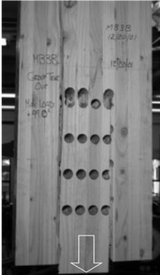
closely spaced fasteners in group tear-out
